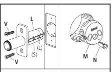
Adjust backset on **L** for door, 2<sup>3</sup>/8" (S) or 2<sup>3</sup>/4" (L). Insert **L** through edge of door deadbolt hole and fasten to door with **V** wood screws. Insert **M** into 2<sup>1</sup>/8" bore and fit **N** into **M**.
