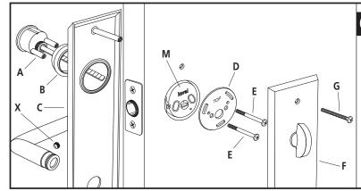
Slide A through B and C and then slide tailpiece through hub of M and large hole of D. The lever attached to the backplate needs to slide onto the spindle in hole below. From interior side, insert the two E screws through D and M and tighten into A. Attach F so that the tailpiece slides into the turnpiece and the spindle below slides into the lever attached to the backplate. Fasten at both ends of backplate using G screws. On both sides of door, secure levers with set screw X.
