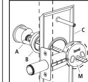
B Slide A through B and C and then insert end of tailpiece into hub of M. Test fit length of tailpiece into F on other side of door to determine where to trim the tailpiece.
