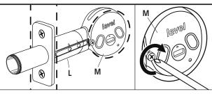
While **M** is inside of 2<sup>1</sup>/8" bore, attach **L** to **M** using screw already assembled to body of **M**.
