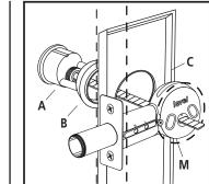
A Slide A through B and C and then insert end of tailpiece into hub of M. Test fit length of tailpiece into F on other side of door to determine where to trim the tailpiece.
