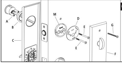
Slide A through B and C and then slide tailpiece through hub of M and large hole of D. From interior side, insert the two E screws through D and M and tighten into A. Attach F so that the tailpiece slides into the turnpiece and the spindle below slides into the lever attached to the backplate. Fasten at both ends of backplate using G screws. On interior side of door, secure lever with set screw X.
