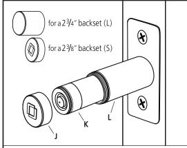
7 Insert battery **K** into deadbolt **L** and thread the correct **J** cover for backset onto deadbolt.
