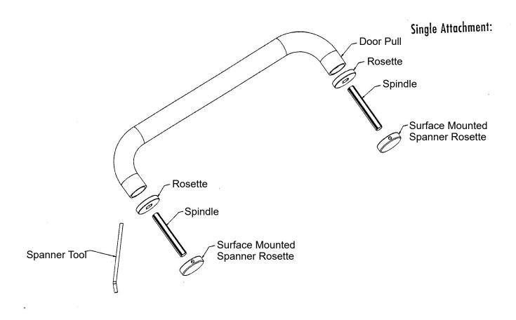
Assemble parts according to exploded view. Spindle fits through hole in door and protrudes on both sides. Affix the Surface Mounted Spanner Rosette to the end of Spindle on opposite side of door from the Door Pull. Insert the Spanner Tool in the hole on the side of the Surface Mounted Spanner Rosette and turn to tighten the assembly.
