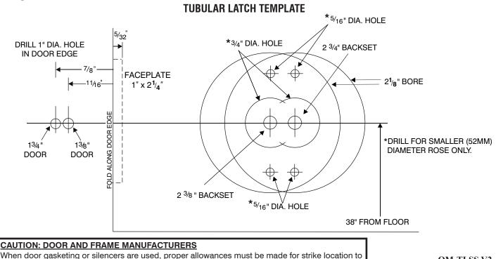
maintain a common centerline with lock and door so that the bolt will freely enter strike.
