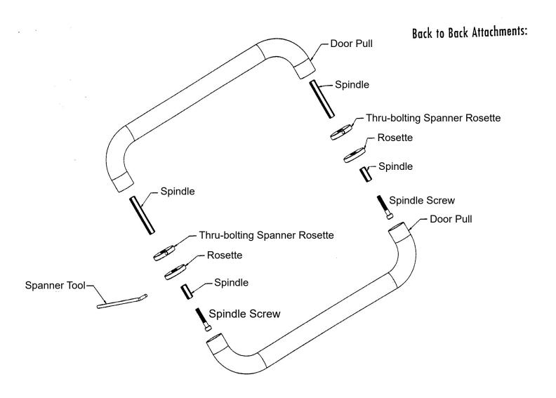
Assemble parts according to exploded view. Door surface is between the thru-bolting spanner rose and the rosette. Position the Spanner Tool in the hole on the side of the Thru-bolting Spanner Rosette and turn to tighten the assembly.
