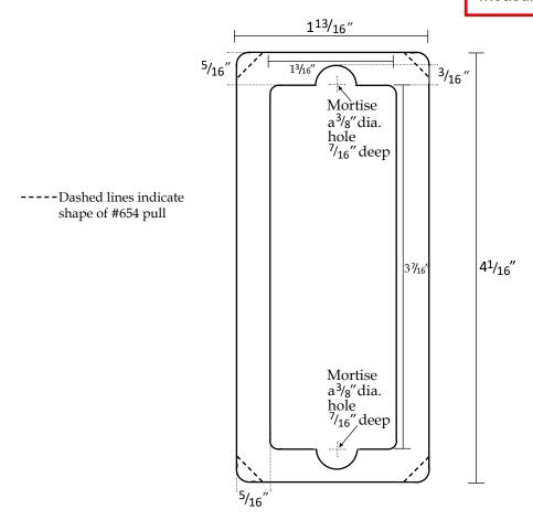
Mortise 37/16'' long x 13/16'' wide x 7/16'' deep. Use brads provided to attach pull to door through the holes at both ends inside the recess.
