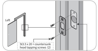
Make sure the hole in the door frame is drilled a minimum of 1"(25mm) deep.
